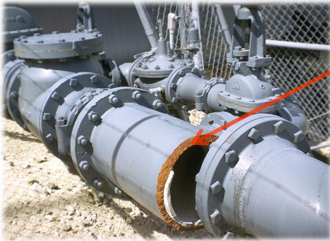
Example of ground piping failure
